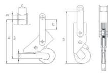
The Automatic Hook is available in 5 sizes from 2 to 20 tons. It is easy to operate, has rugged design and a high reliability.
